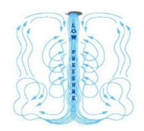
The system has a natural de-stratification effect. Warm air that normally rises and is lost at ceiling level is redistributed downwards to where it is needed at floor level. This means that temperatures are even, with no hot/cold spots.
